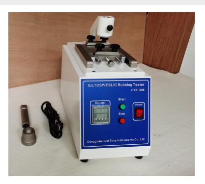
specifications Rubbing finger: 500 +/- 25 g(or 1000g by adding a load mass) Loading weight: 500 +/- 10 g Dimension of base of finger: 15 x 15 mm Specimen: 120x20mm Rubbing stroke: 35 ~ 40 mm Speed of rubbing: 40 +/- 2 cycles/min Counter: LCD,1-999,999 times, automatically stops Instrument Weight: 35kg Power: 220/110 V,50/60 Hz,4A
