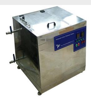
Put the tested specimen, steel ball and detergent together into the test cup. Scroll through the spindle to make friction between the sample and steel ball.
