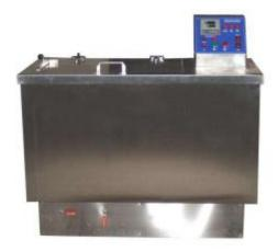
Put the tested specimen, steel ball and detergent together into the test cup. Scroll through the spindle to make friction between the sample and steel ball.
