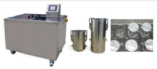
Put the tested specimen, steel ball and detergent together into the test cup. Scroll through the spindle to make friction between the sample and steel ball.
