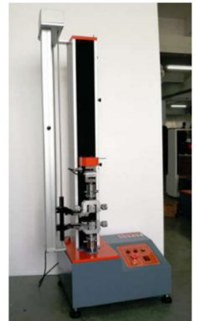
HTP-001B Computer Control with extensometer
