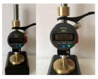
Main Parameters: Micrometer Brand: Mitutoyo, Japan Range: 0-12.7mm Graduation: 0.001 mm ((1μm)) Throat depth: 150mm Total Accuracy: ± 3μm Contact Point Dia: 6±0.05mm Parallelism: <0.005mm (5μm) Applied force: 0.5-1.0N Table base size:150mm\*100mm
