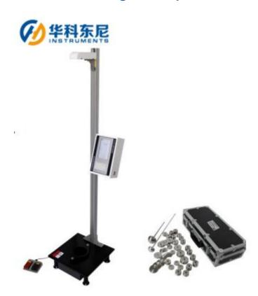
**Application :** For the determination of the energy causes the plastic film to fail under specified conditions of impact of a free-falling dart.
