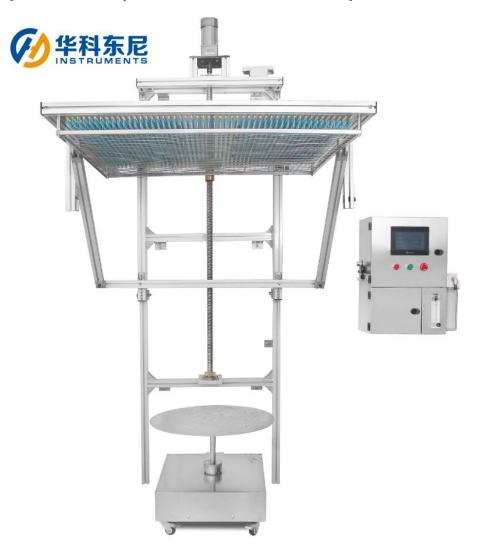
**Principle:** Simulate the damage of natural water (rain, seawater, river water, etc.) to products and materials, and waterproof testing of product casings.
