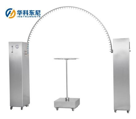
**Principle:** Simulate the damage of natural water (rain, seawater, river water, etc.) to products and materials, and waterproof testing of product casings.
