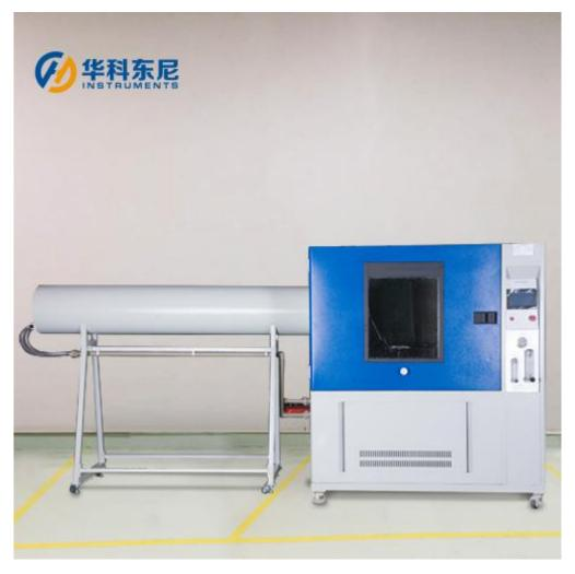
**Principle:** IPX5 IPX6 Water Jetting Test Chamber is applied to test the water tightness of enclosures of automotive parts, outdoor lamps and electronics parts.
