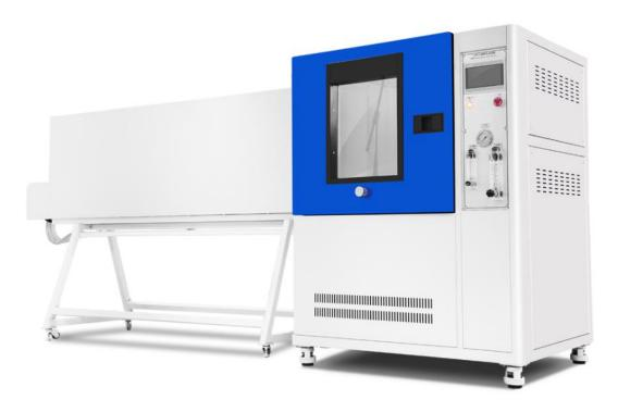
**Principle:** IPX5 IPX6 Water Jetting Test Chamber is applied to test the water tightness of enclosures of automotive parts, outdoor lamps and electronics parts.
