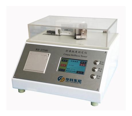
The RH-ZT500 crease stiffness tester is mainly used for the determination of indentation stiffness (rebound force of 90 ° folded) for various cardboard and cartons such as cigarette boxes. It is used to judge the folding performance of various cardboard or cartons. At the same time, it can also be used for the determination of various cardboard bending stiffness. With two-point loading, it is an efficient and easy-to-use instrument.
