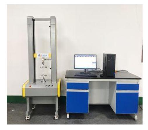
This machine/Tensile Strength Testing Machine is suitable for rubber, tires, hoses, tapes, soles, plastics, films, acrylic, FRP, ABS, EVA, PU, aluminum-plastic pipes, composite materials, waterproof materials, fibers, textiles, wires and cables, paper, gold foil, tapes, silk threads, springs, wood, pharmaceutical packaging materials, tapes, etc. for tensile, compression, tearing, peeling (90 degrees and 180 degrees) and other mechanical properties test and analysis.
