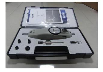
Imada Pointer Push-Pull Force Gauge is a small and simple thrust and tensile force testing instrument. It is suitable for push and pull load test in electronic appliances, light industry and textile, hardware, lighter and ignition device, fire fighting equipment, manufacturing, fishing gear, power machinery, scientific research institutions and other industries. It is a new generation of products that replace tubular push-pull force meters.
