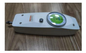
Pointer push-pull force meter is a small and simple thrust and tensile force testing instrument. It is suitable for push and pull load test in electronic appliances, light industry and textile, hardware, lighter and ignition device, fire fighting equipment, manufacturing, fishing gear, power machinery, scientific research institutions and other industries. It is a new generation of products that replace tubular push-pull force meters.
