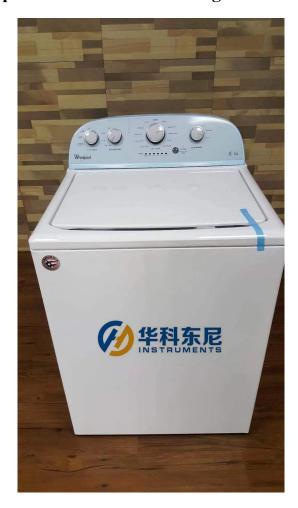
Whirlpool 3LWTW4815FW 15kg AATCC Washer.AATCC standard washing machine is a standard water shrinkage tester specified by AATCC in the United States, which meets the AATCC testing standards method. AATCC standard washing machine washing textiles one time equivalent to the shrinkage or elongation of household washing machines after washing textiles many times, which can be used to evaluate the appearance of textile after washing.
