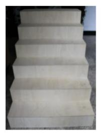
This instrument is mainly used to tumble test for Wheeled toys weighing more than 3 lb (1.4 kg) but not more than 10 lb (4.5 kg). Standards: ASTM F963 section 8.7.3.
