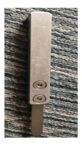
EN 71 Feeler Gauge is used to determine whether parts on toys can be stepped up so as to determine whether the tensile testing is necessary.
