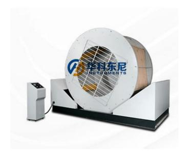
This machine imitates the damage test of suitcases and other packaging boxes during transportation, such as dropping, impact, and rolling, and tests the protection ability of suitcases and contents, as the basis for product improvement.
