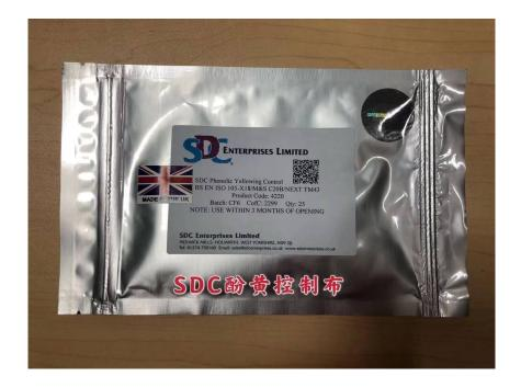
SDC Phenolic Yellowing Control-25 Pcs/Bag are used to assess the probability of yellowing of textiles during transport and storage. Suitable for white or light-coloured yarns, fabrics or finished garments.
