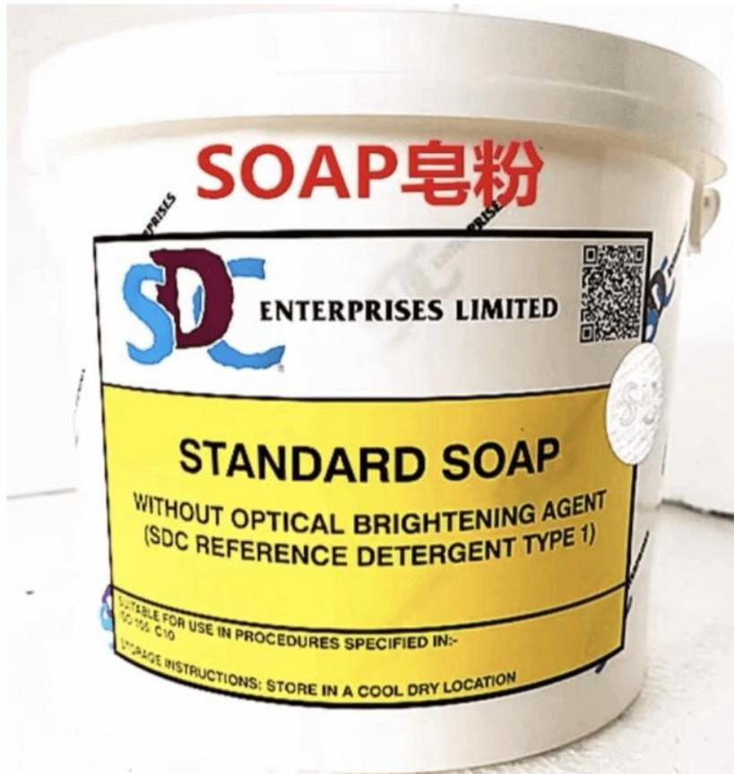
SDCE Standard Soap (SDCE Type 1). This product is manufactured for use in the ISO 105 C series of Colour fastness tests.
